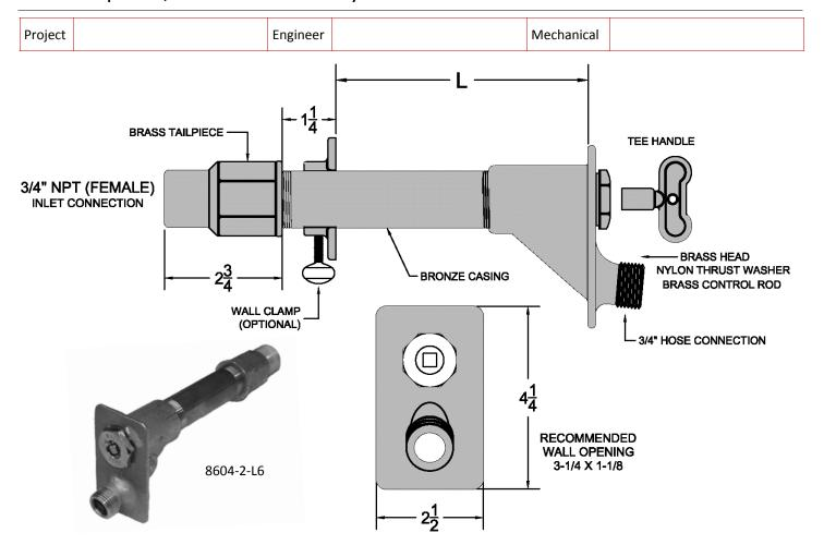
**Regularly Furnished:** Non-Freeze wall hydrant with compression closure valve, bronze casing, 3/4" hose connection.
