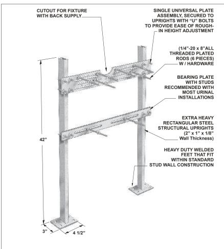
MC-32 Series Meets ANSI/ASME fixture carrier standard A112.6.1M-97
