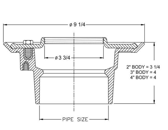
**SPECIFICATION:** JOSAM 30000-PVC SERIES PVC FLOOR DRAIN, TWO-PIECE BODY WITH DOUBLE DRAINAGE FLANGE, 1/2" PRIMER TAP WITH PLUG, WEJLOC INVERTIBLE NON-PUNCTURING FLASHING COLLAR WITH WEEPHOLES, SOLVENT WELD BOTTOM OUTLET FOR SCHEDULE 40 PVC PIPE, AND THREADED TO RECEIVE ALL JOSAM ADJUSTABLE STRAINERS.
