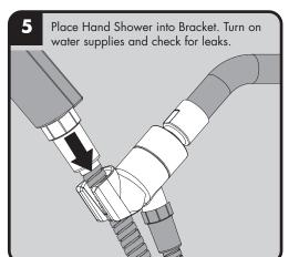
Ensure Hose Washer is inserted inside connector to avoid leaks. Thread Hose End with Label to the outlet port of Bracket. Hand tighten.
