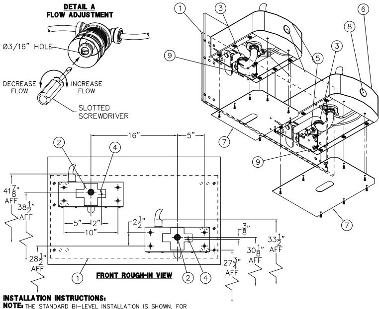
NOTE: THE STANDARD BI-LEVEL INSTALLATION IS SHOWN. FOR OPTIONAL -RBL REVERSE BI-LEVEL CONFIGURATION, THE INSTALLATION IS OPPOSITE TO THAT SHOWN.
