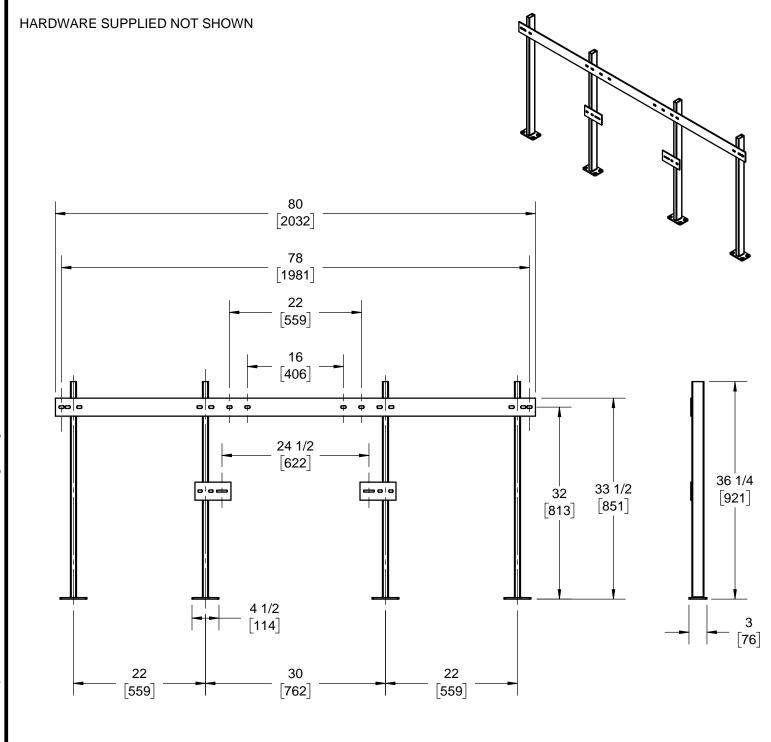
RECOMMEND FEET TO BE SECURED TO FLOOR WITH 1/2" BOLTS AND ANCHORS BY OTHERS.
