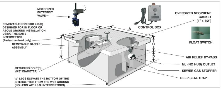
**Note:** The "C" dimension detailed above is from either the middle of the inlet or the outlet to the top the interceptor. The inlet and outlet dimensions are always the same.
