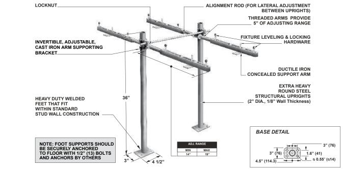
MC-41D-R Series Meets ANSI/ASME fixture carrier standard A112.6.1M-97
