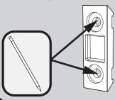
If mounting directly to wood stud, Plastic Anchors are not required. If mounting to drywall, drill guide holes at marked locations using a Drill equipped with a Ø 3/16" bit.
