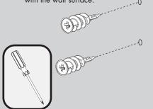
Secure Mounting Plate with the Mounting Screws provided. Verify that the Mounting Plate is aligned vertically.
