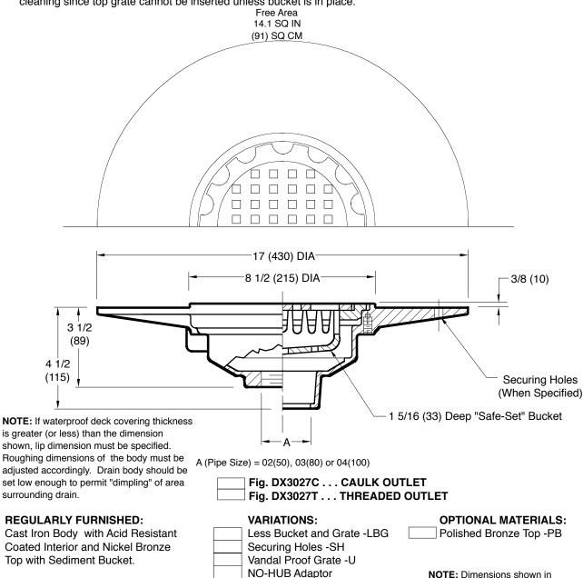
Cast Iron Body with Acid Resistant Coated Interior and Nickel Bronze Top with Sediment Bucket.
