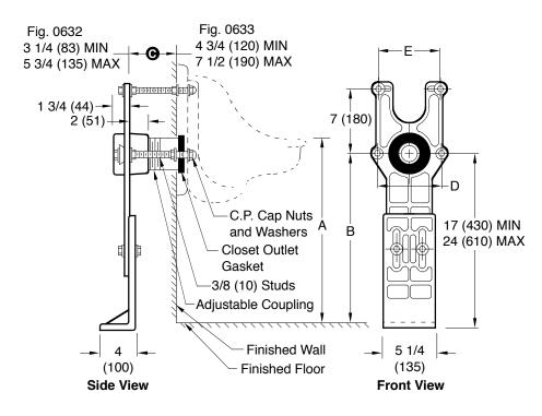
Fig. 0632 . . . 2" (50) Outlet Connection Fig. 0633 . . . 3" (80) Outlet Connection
