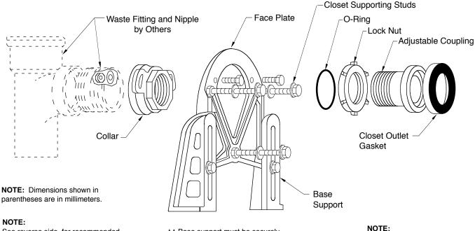
Δ See reverse side for recommended setting of closet outlet connection and various modifications.
