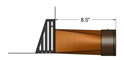
16 oz copper flashing soldered to spout, attached to 2", 3", or 4" bronze no-hub fitting
