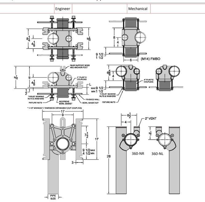
Regularly Furnished: Fixed, offset vertical water closet carrier with 2" vent, floor mounted foot supports, & faceplate.
