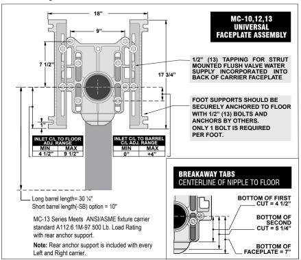
Note: 8" tapered thread ABS nipple shipped standard with MC-13 Series carriers. The universal faceplate assembly accepts all nipple variations, rolling thread (-OR), cast iron (-Cl) and tapered thread ABS with adjustable horn (-AH).
