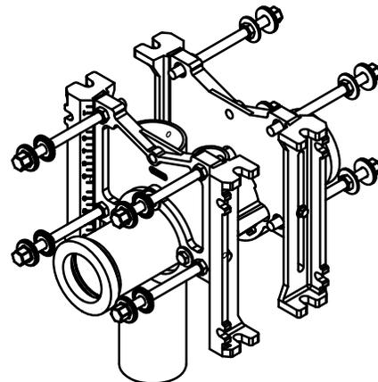
FOR 2" NO-HUB AUX. INLET, EITHER CUT IN FIELD OR SPECIFY (-50) THREADED (-54)
