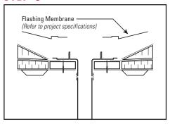
Caulk the outside edge of the drain with compatible water cut-off or roofing cement.
