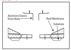
Cut hole in deck 2-in. larger than the outside diameter of the drain stem being installed. Create a new base plate made of plywood that extends 2-inches beyond the drain flange. Carefully align hole in base plate with hole in roof deck and secure in place. Taper insulation to the edge of the base plate.
