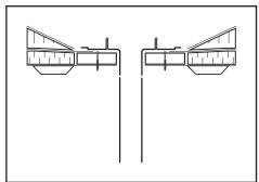
Attach appropriate length tail piece of drain pipe with the mechanical connector provided. Center drain in hole and fasten to base plate; screws should be installed through the raised outside edge only.
