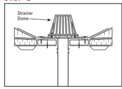
Install clamping ring and strainer dome. Connect drain to interior plumbing pipe with mechanical connector provided.
